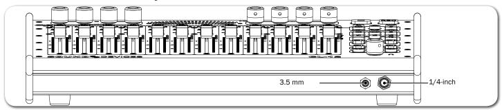
The back panel provides the two connections required (USB and Headphone) for attaching the CL-12 to the 688, plus ports for other peripherals.
