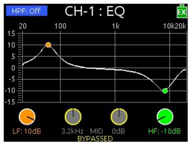
It is not possible to adjust EQ for multiple inputs at the same time. When multiple input channels are selected, the channel that is adjusted will be the last one added to the group.
