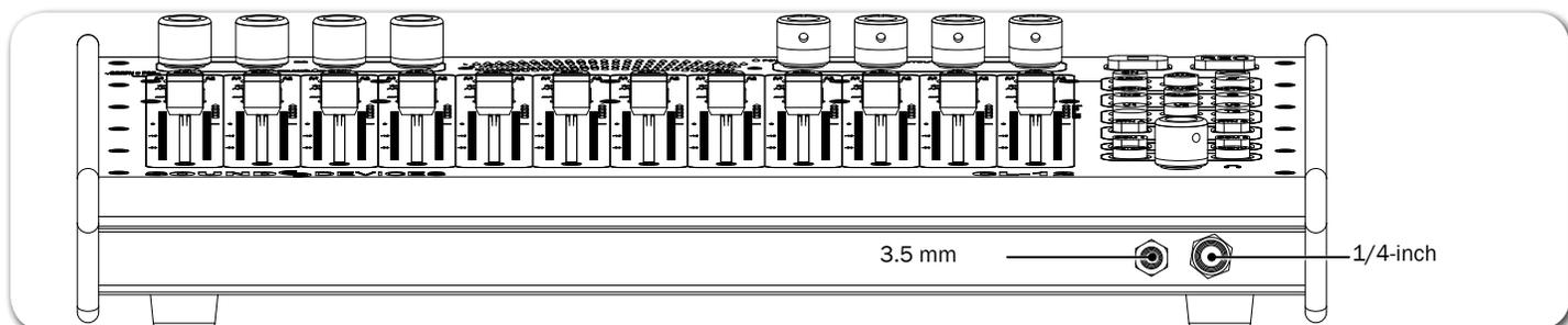
The back panel provides the two connections required (USB and Headphone) for attaching the CL-12 to the 688, plus ports for other peripherals.
